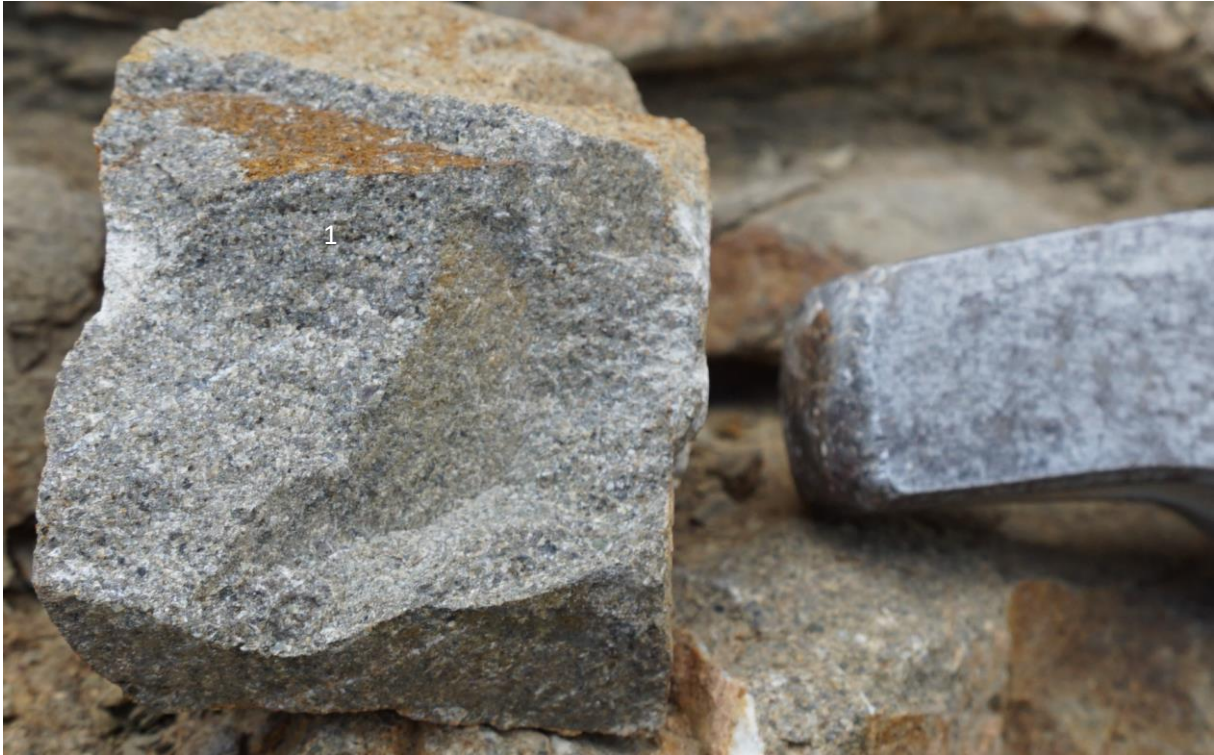
1: Closeup of the sandstone, which is probably a greywacke, due to its content of different immature clasts and lithic components. The greywacke represents material deposited by a turbidity current.
